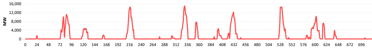
Battery Energy Storage Deployed During Modeling Period
